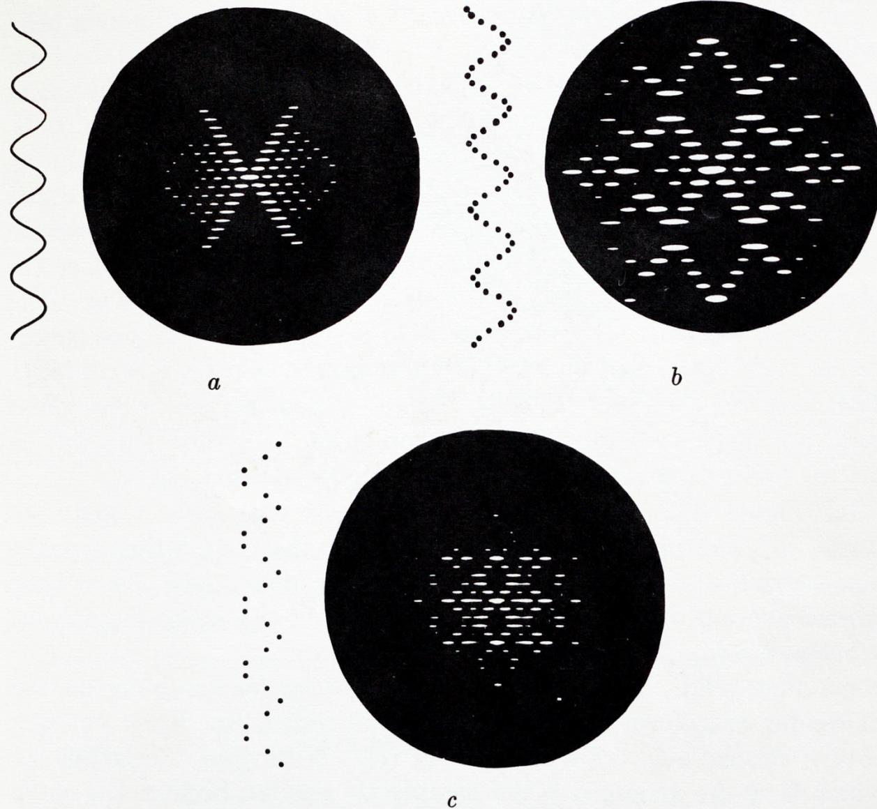
Fig. 32. (a) Optical transform of a continuous helix. (b) Optical transform of a helix with 10 points per turn. (c) Optical transform of a helix with 5 points per turn.
