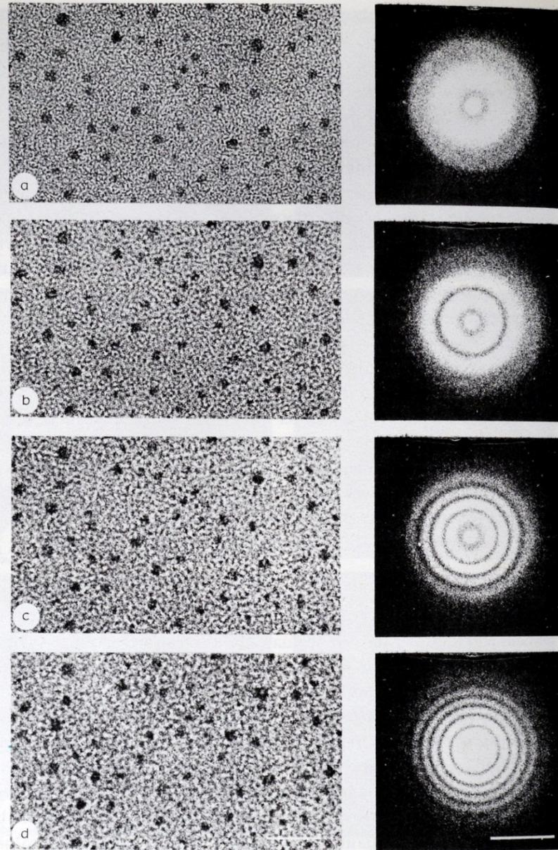
Fig. 3.8. Focus series of a thin carbon film, plus gold particles to assist in focusing. The optical diffractograms are alongside each image: (a) optimum defocus, (b) 150 nm underfocus, (c) 210 nm underfocus, (d) 250 nm underfocus.  $C_s$  and  $\Delta f$  are determined by measuring the radii (or diameters) of the dark circles corresponding to minima in the optical transform.  $E_0 = 125$  keV, image bar = 10 nm, diffraction bar =  $3.0 \text{ nm}^{-1}$ . (P. Sieber, unpublished.)
