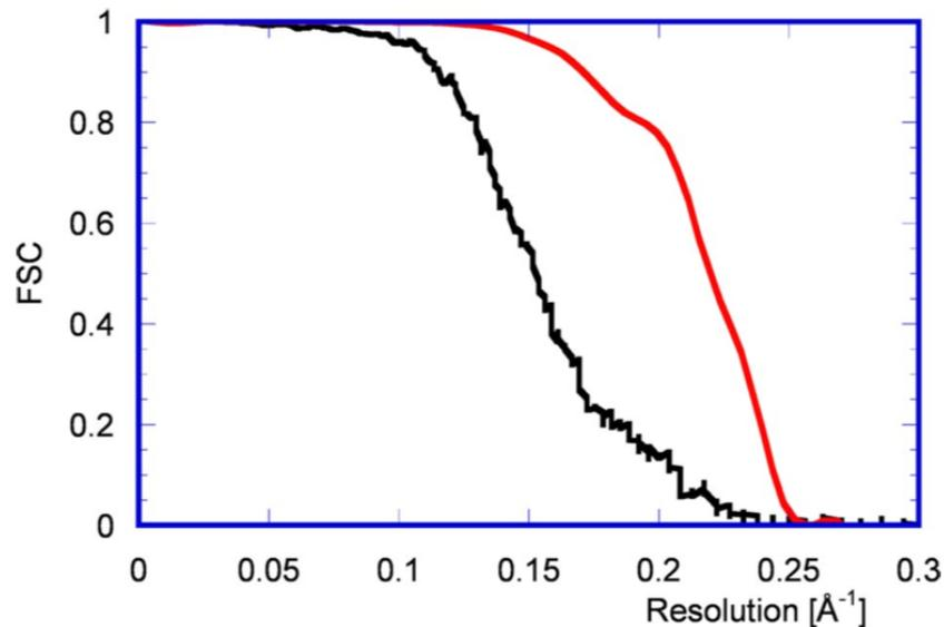
**Fig. 4.** FSC curves before (black) and after (red) 13-fold nonicosahedral averaging. The black curve suggests a resolution of 5.1 Å (0.143 threshold value), and the red curve indicates a resolution of 4.1 Å.
