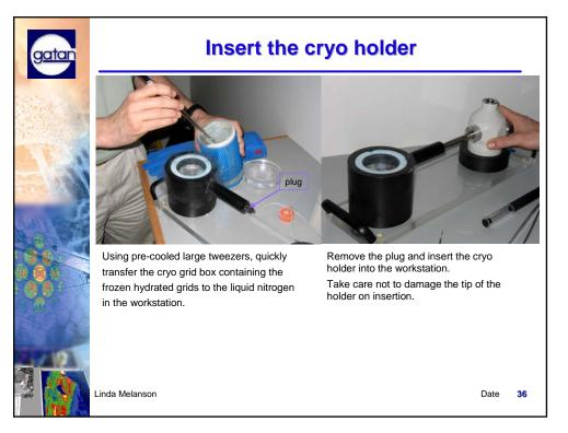
Once the specimen grid box is in the workstation, load the holder by removing the black plug (which is held in place via an o-ring seal – so remove it by just pull the plug straight out from the arm of the workstation.)
