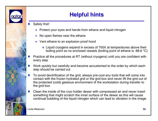
Liquid cryogens expand in excess of 700X at temperatures above their boiling point so no enclosed vessels (boiling point of ethane is -88.6 °C) and no sources of ignition in the area where the plunging will take place.
