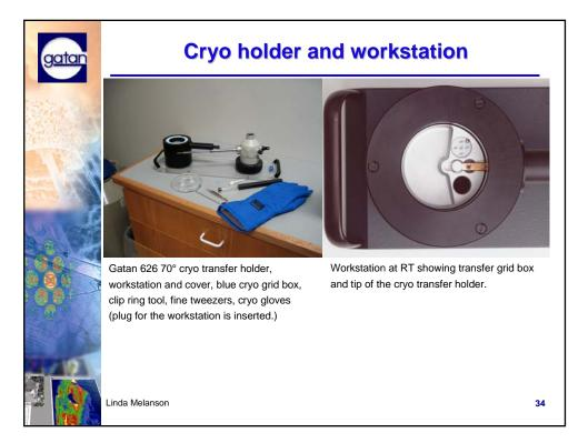
Close-up of the Gatan 626 70° cryo transfer holder and workstation.
