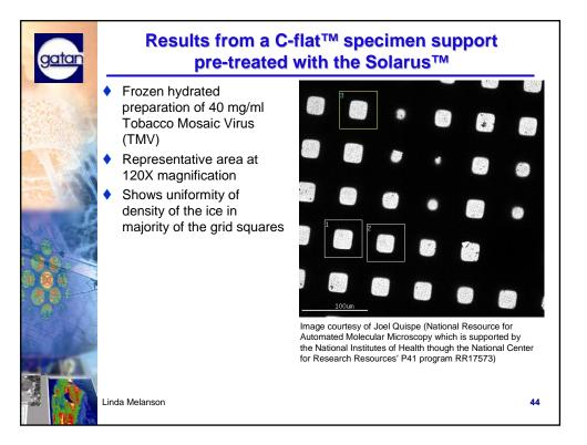
This image is the first in a series of images showing a grid pre-treated with the Solarus to make it hydrophilic and then plunge frozen in liquid ethane and viewed on an electron microscope under low electron dose conditions.
