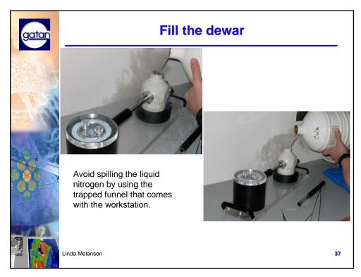
Quickly fill the liquid nitrogen dewar of the holder to get it to temperature. The tip will cool down immediately once it is inserted into the cool environment of the workstation. There are many
