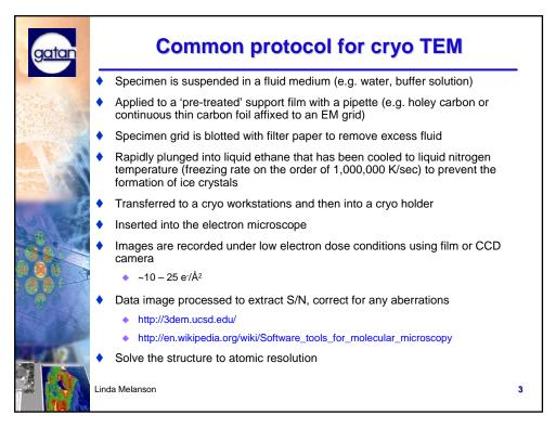
There are many different ways to prepare a specimen for viewing via cryo methodologies. This talk will only look at methods that center around specimens that are suspended in an aqueous medium and that can be blotted and plunge frozen in liquid ethane and then viewed, using low electron dose techniques, on a TEM.
