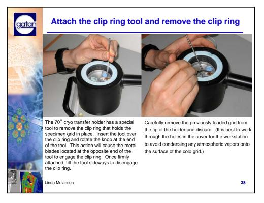
For the purpose of observing what is happening within the workstation chamber, the workstation cover has been removed for the following images. Normally, one would work with the cover in place, working through the two opening in the cover in order to protect the specimen from condensation of atmospheric vapor (and subsequently the formation of frost) onto the surface of the grid.
