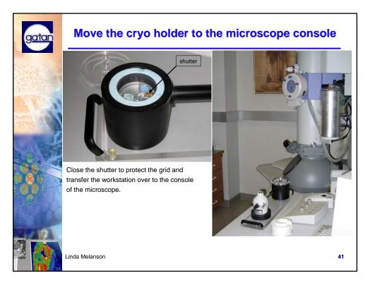
• Close the shutter to protect the grid and transfer the workstation over to the console of the microscope. You want to minimize the transfer of the grid in room air even though it is protected by the cryo shutter so it is best to move the entire workstation with holder and grid to the microscope console.
