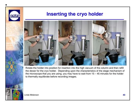
Following manufacturer's directions for your particular electron microscope, insert the holder into the airlock. Rotate the holder into position for insertion into the high vacuum of the column and then refill the dewar for the cryo holder. Depending upon the characteristics of the stage mechanism of the microscope that you are using, you may have to wait from 15 – 45 minutes for the holder to thermally equilibrate before recording images.
