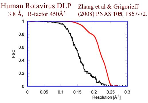
**Fig. 4.** FSC curves before (black) and after (red) 13-fold nonicosahedral averaging. The black curve suggests a resolution of 5.1 Å (0.143 threshold value), and the red curve indicates a resolution of 4.1 Å.
