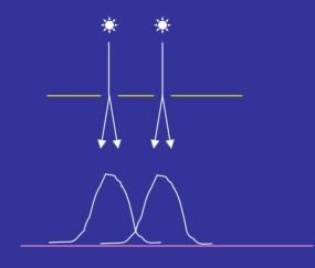
The resolution of a microscope objective is defined as the smallest distance between two points on a specimen that can still be distinguished as two separate entities.
