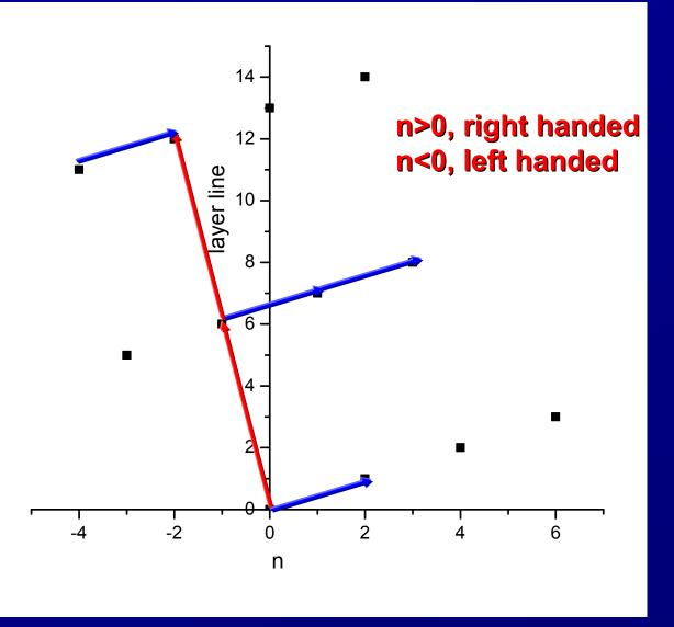
n,l plot is reciprocal lattice of helical net each point corresponds to n-start helix, pitch=|n|\*c/l infinite number of points, infinite number of helices! we can understand n,l plot in terms of diffraction from helical objects projection of a single helix is a sinusoid Fourier transform of helix generates "layer lines"
