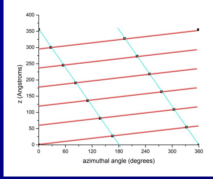
There are an infinite number of different helices that pass through subunits
